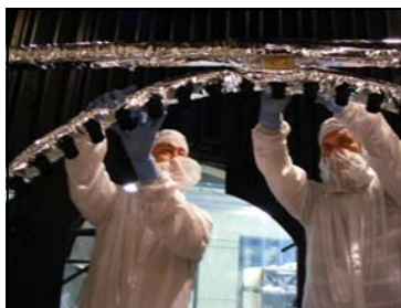
Mike Lynch and Chad Sheng installing the Baffle Test Fixture in the Thermal Vacuum Chamber.
